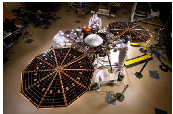
The solar arrays on NASA's InSight lander are deployed in this test in a clean room at Lockheed Martin Space, Denver, in April 2015. Each of the two arrays is 7.05 feet (2.15 meters) in diameter.
